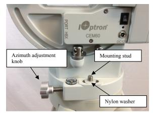
Figure 14. Attaching the mount
